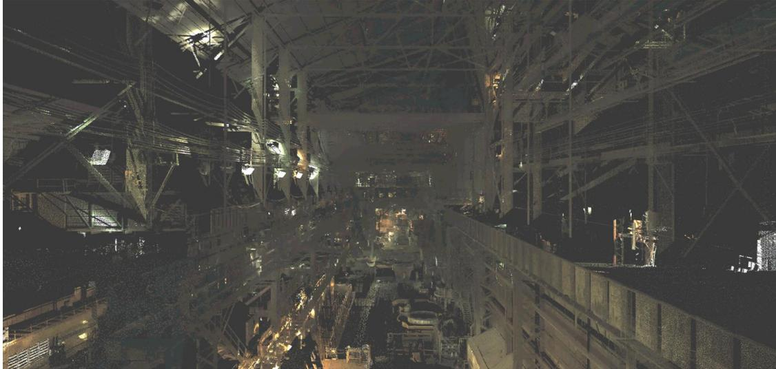
\*Screen shot of laser scanner output. Each pixel represents 3D measurement.
