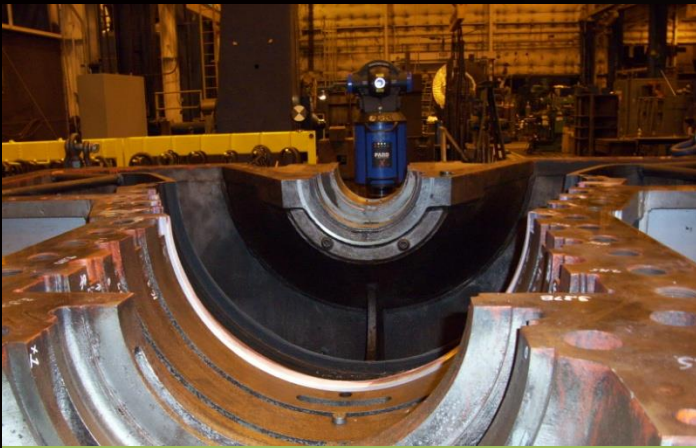
Picture 1: Utilizing laser tracker technology for bore alignment.
