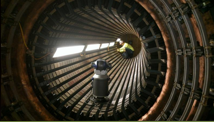
Picture 1: Using a laser tracker to verify concentricity of magnetic plates on stator unit.
